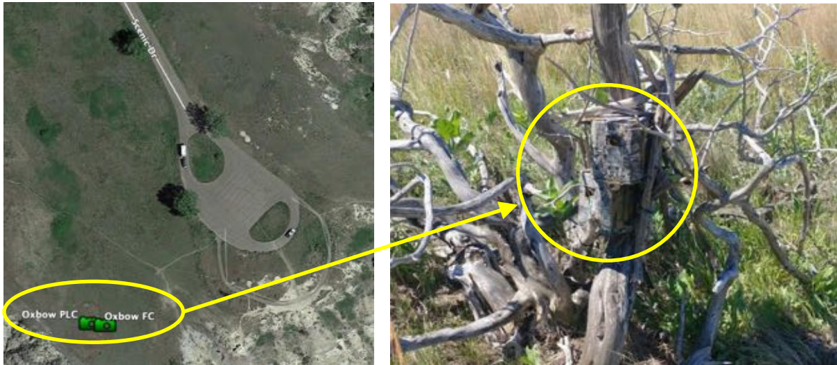
Figure 78. At the Oxbow Overlook parking lot, researchers placed two wide-angle Spypoint cameras to capture both field activity (not presented due to damage) and parking lot activity. The PLC faced northeast toward the parking lot. Both cameras were mounted to the base of a dead tree. Equipment coordinates in Appendix X.
